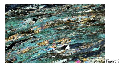
ii) Nematoblastic Texture-Abundant linear minerals (actinolite, hornblende, etc.) with strong preferred orientation (Causes Lineation). (Figure 8- Nematoblastic glaucophane)
